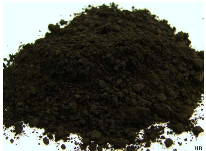
Also called burned sheep bones and burned stag horn. These are some of the finest polishes. The bones or horns are burned with only a little oxygen and the leftover ash is used as an abrasive or pigment and consists largely of phosphoric calcium.
