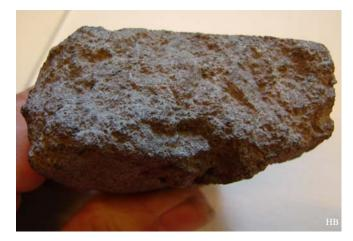
On the emery stone at the paint-mill "De Kat": This is a very hard rock from the Greek island of Naxos. This was not used as a dye but for grinding and polishing purposes.
