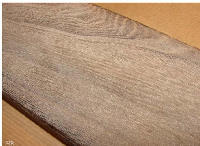
This macro shot shows how the abrasive grains have sunk into the surface of the wood.
