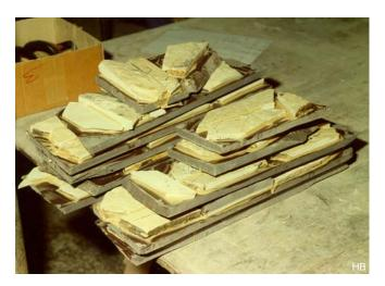
The coticule not always comes with a sufficiently thick layer of blue-violet "Rouge de Salm". Using Araldite (2 comp. Epoxy glue) it is glued to a piece of Rouge de Salm. In ancient times Lorraine was used. Rouge de la Salm also has a very good grinding effect by the garnet grains (in the amount of 20 to 40 microns) contained therein.
