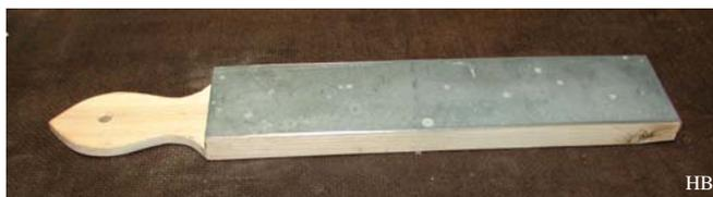
We had to try out this method. A cut off of ash was cut in the form of the test-paddles and a piece of zinc put on top. The result is very surprising. It provides a frosted surface. Clearly an example of the operation called 'lapping'. The Emery grains roll over the zinc and occasionally tap a small part from the material. This contrasts with the grinding operation that causes grooves. After that a chisel was sharpened and I also got surprisingly sharp results, with a long service life.
