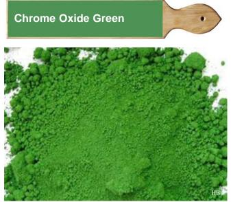
Chromium oxide (Cr2O3), has the structure of aluminum oxide, and consists of a hexagonally packed array of oxide anions with 2/3 of the octahedral holes covered by chromium. Similar to aluminum oxide, chromium oxide is a hard and brittle material (Mohs hardness 8-8.5). It is brown when heated but returns to its dark green colour when cooled. It is hygroscopic.
