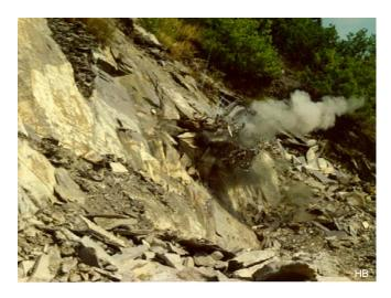
The raw material in the quarry is made loose by using black powder and brought from the quarry to the workshop for further processing.
