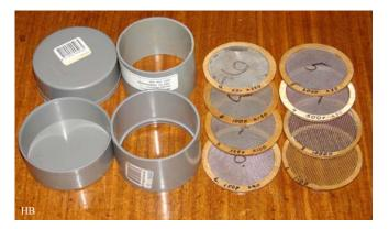
With some tinkering, aircraft plywood, epoxy glue and drainpipe we have made ourselves a useful sieve set. The series now runs through 1100, 1000, 800, 300, 200, 150, 125, 100 and 65 microns.
