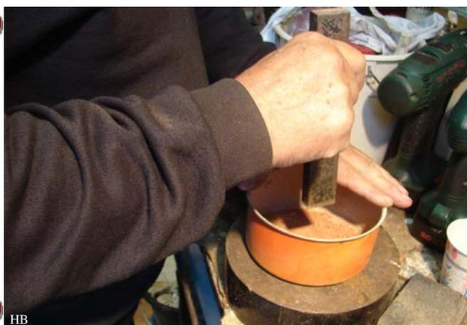
Since we have no biksteen or paint mill at our disposal, we have pounded to powder with particles smaller than 300 microns (K54), a Groningen brick made by Strating and an old Dutch tile from Uitgeest (made from clay with a different origin), using a rod of iron in a saucepan over a 6 cm thick steel plate.
