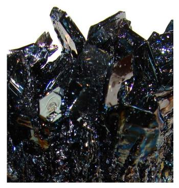
SiC is used for grinding and polishing, in the form of grinding wheels, polishing and abrasive powders and as coating of sandpaper. It is produced industrially by Kollo Silicon Carbide in Delfzijl. The density is  $3.22 \text{ g} / \text{cm}^3$ . The hardness = 9.5 on the Mohs scale (diamond 10) and it is resistant to high temperatures, acids and bases. If it is broken down sharp points emerge again.
