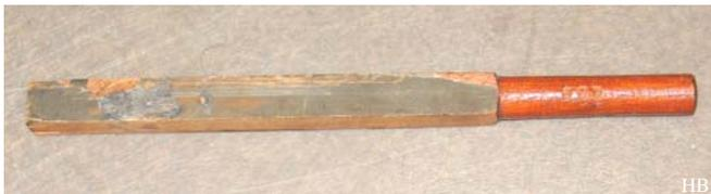
In the years 1958-1961 I trained as an instrument maker. Here we used a wooden abrasive file with very fine waterproof sandpaper glued on. The file was made from a piece of teak with a turned round handle. As a glue we used heated colofonium resin.
