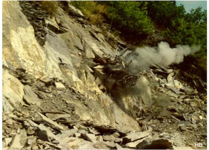
The raw material in the quarry is made loose by using black powder and brought from the quarry to the workshop for further processing.
