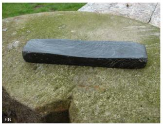
A broken sandstone grinding wheel with a prewar Thuringian whetstone on top.
