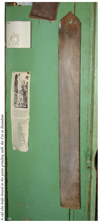
The old original knife-boards show that they are used and therefore become thinner in the middle. The used ones also show that a part of the grains have been pressed in the wood and thus grind instead of "lapping".
