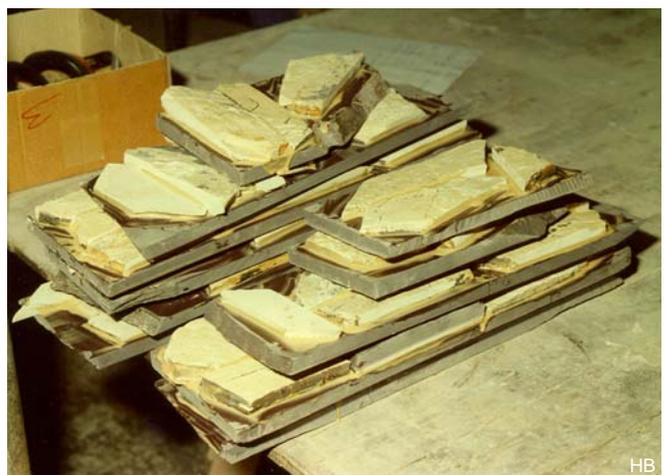
The coticule not always comes with a sufficiently thick layer of blue-violet "Rouge de Salm". Using Araldite (2 comp. Epoxy glue) it is glued to a piece of Rouge de Salm. In ancient times Lorraine was used. Rouge de la Salm also has a very good grinding effect by the garnet grains (in the amount of 20 to 40 microns) contained therein.
