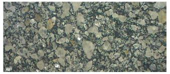
Biksteen fine, particles <54. With this we will do the honing test.
