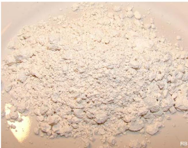
Vienna lime (or Weener Lime) is a special kind of pure lime, which is entirely free of aluminum, iron and magnesium oxide. Because it is very fine, soft and pure it lends itself well to make cleaning and polishing materials.
