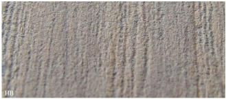
Very fine particles biksteen are in the pores of the wood.
