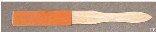
Another skill was making technical drawings where a knife-board was used to give the pencil a nice sharp point and to make a nice bevel on the pencil lead of the compass. It was the era that we had no Red Ring Pens and pencils, but we were using a poplar drawing board and beech drawing hook.
