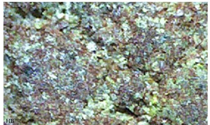
The characteristic of a grinding stone is that the pressure on the grains is not equal in size. This means that not all grinding grooves are of the same depth. Its depth depends on the size of the grains and the applied pressure.
