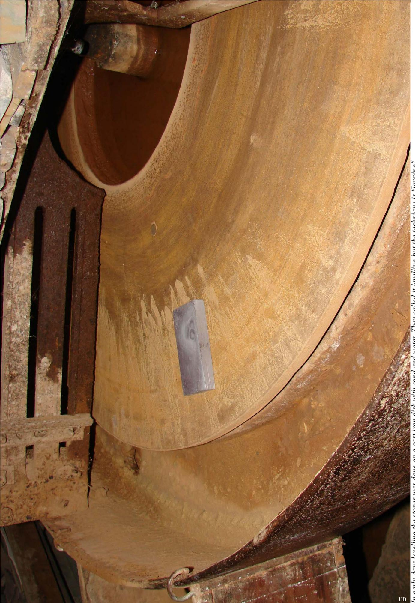
*In early days levelling the stones was done on a cast iron disk with sand and water. They called it levelling but the technique is "lapping". Nowadays the stones are levelled on a diamond disk.*
