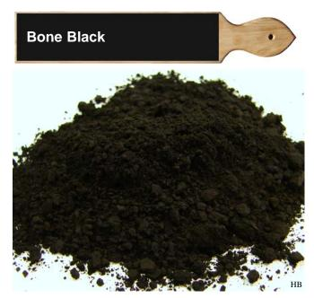
Also called burned sheep bones and burned stag horn. These are some of the finest polishes. The bones or horns are burned with only a little oxygen and the leftover ash is used as an abrasive or pigment and consists largely of phosphoric calcium.
