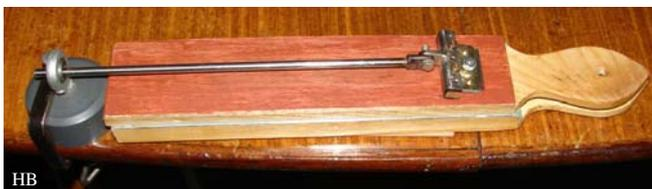
In this the blade stretches out further and the blade holder can be taken off. This piece is ground off underneath to produce a 10 degree sharpening angle. The blades are 0.1 mm thick and the cut is 0.3 mm long...
