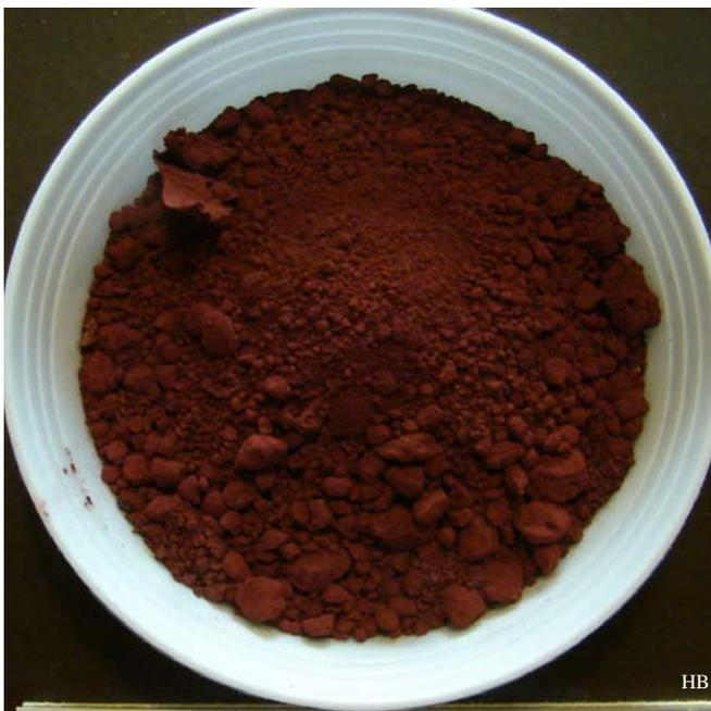
Colcothar is a red and purple dye, almost entirely consisting of iron oxide ( $\text{Fe}_2\text{O}_3$ ) and clay soil. It is an artificial mineral pigment. It is extracted from weathered iron ore rock or clay by a process of washing and grinding. Colcothar contains about 87% iron oxide and only 10% English Red. These pigments have been used since the ice age.
