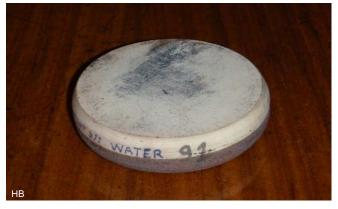
A round, in this case artificial corundum sharpening stone used in machine technology. Similar to the stone used for axes. The name is also used for a circular grinding wheel for a grinder.
