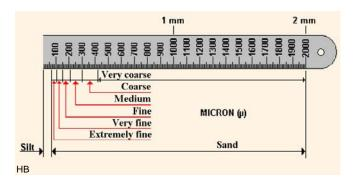
\* The rock is very fine, when the grains are not visible to distinguish to the naked eye. Than the grains are smaller than 0.065 mm. It is a microscopic rock. For whetstones this applies for instance among others to slate.
