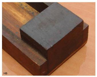
Sometimes at the beginning and the end of the stone a piece of wood is placed which is the same height as the stone so when the grinding the cutter a longer stroke can be made.
