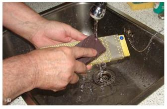
The DMT can be kept loose by hand. In this way it is easy to make a circular motion, and the result is perfect.
