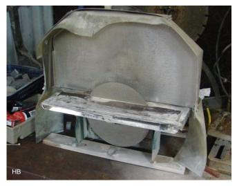
During a visit to a whetstone maker I've seen this grinder. The green part was familiar to me as part of a tile saw. During our conversation about the grinder I got a used 8 inch (200 mm) "electroplated diamond grinding disc" to try it out.
