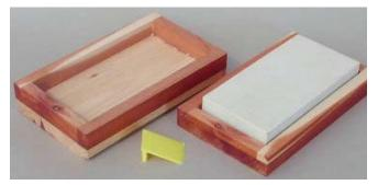
Simple construction of cedar. The stone is loose.
