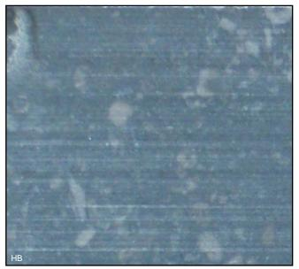
C220 = Slightly honed: fine grinding, colour and structure clearly recognizable, grinding marks still visible in raking light.
