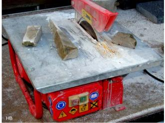
\* Tile Saw to cut perpendicular sides.
