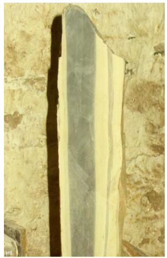
Coticule alternating with shale is easier sawing.
