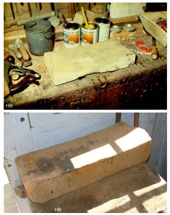
2) Is in one way or another the edge of a chisel got blunt, then it is sharpened on a sandstone, which grit may be not too fine nor too coarse. Sometimes a sliding stone is used instead of a whetstone. Sliding stones usually have a more or less rectangular shape. They can be purchased at a hardware store, but usually one can get a discarded piece of a grinding stone at be a carpenter.
