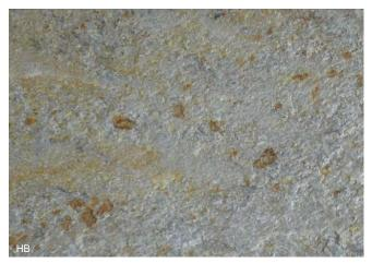
Pyrite inclusions are sometimes found in Thuringer whetstones are no danger to the object to be sharpened. Pyrite is soft and will not damage the cut even though they sometimes break out and take with it grains that may do damage. Pyrite is also called "fools gold".
