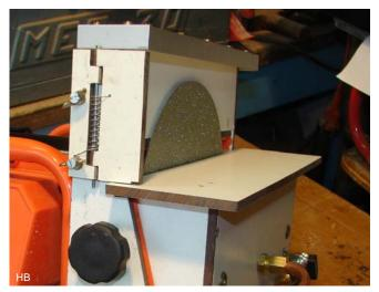
The diamond discs should be water-cooled to ensure that the disk will last long. There is needed very little water and the speed creates a mist of water. In order to prevent the water from being thrown far away, there is arranged a spring-loaded valve so that even long stone can be grinded. Without valve the water came up to 2 meters.
