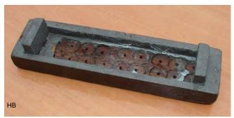
How you make the cavity in the wood depends on your tools. Previously this was done with a centre wood bit, but now I should use a router.
