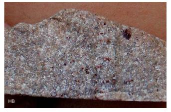
In sandstone arisen through metamorphosis, the bond between the grains is weaker so the blunt granules break out and new abrasive grains are on the surface again. Yet we can greatly benefit from silica in fine whetstones: we can use it for the last strokes to polish the cut. The fineness can be very high.
