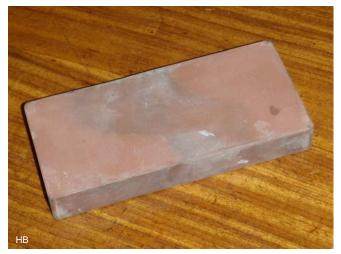
Water stones produce the best cut in the shortest possible time. For polishing of a cut no oilstone, ceramic or of natural origin cannot compete with a water stone.
