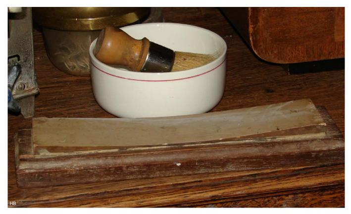
On this stone many razors are sharpened and it is nearing the end of its life. Razors still can be sharpened in this way but not a chisel or planer. You need a flat stone so the cut will be plane.
