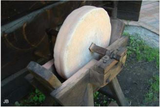
A grinding wheel is a stone-like material to grind or sharpen tools, or to grind anything.
