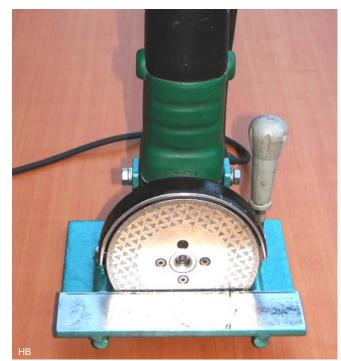
The thickness of the nickel layer is about 50% of the grain diameter. The crystals are thus held firmly but are stabbing from the binding, so a very open granular structure is formed. This disc is very good to use for relatively soft stones like marble and slate. For hard materials a resin bound cup grinding wheel has a longer life, see page 45. Optimum cutting speeds: dry 8 to 18 m/s, wet 15 to 30 m/s. Converted to dry about 1500-3000 rev/min.
