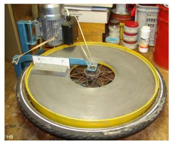
The wheel is mounted in a large steel frame. A 230 V electric engine of 0,25 kW drives the wheel via a 18 mm steel shaft, allowing for a 1:37 speed reduction to make the wheel go round at a pace of about 38 revolutions per minute.
