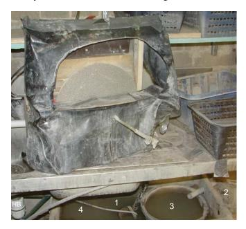
In this arrangement, the water is raised by a submersible pump to the grinder. The return water comes in bucket 2 that overflows in bucket 3, which in turn runs into bin 4. The buckets serve as a settling tanks.
