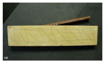
With pencil is a grid drawn on the stone. This allows us to verify the surface of the stone indeed has become flat.
