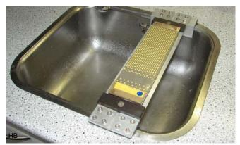
A more convenient way is to make use of a so-called grinding bridge. http://www.amazon.de/Schleifbr%C3%BCcke-Schleifbank-
