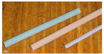
Usually round bar-shaped stones that can be used for inside sharpening of a gouge.
