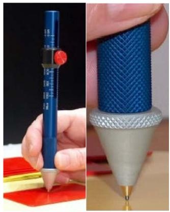
Hardnesspen Labomat of SP0010. A pocket instrument for testing the hardness and wear -/ scratch resistance of the materials. Tungsten Carbide a point is drawn over the surface with a predetermined constant pressure. See: <u>www.labomat.eu</u>
