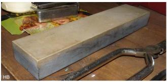
Rectangular stone usually in a box used to sharpen chisels on a workbench. The name is also used for other rectangular grinding- and whetstones.
