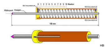
After some pondering, a sketch was made for a homemade sclerometer. Made with a carbide scriber some scratches with the test set of MTN while the stone was on an electronic scale.
