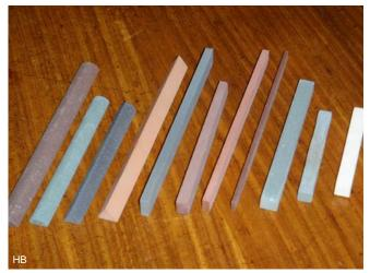
Sharpening files are regularly used by both the jeweller and in machine technology. They exist in natural materials and ceramics made of corundum and silicon carbide. A set consists of coarse, medium and fine in square, triangular, circular, semicircular,  $6 \ge 100$  to  $20 \ge 200$  mm.
