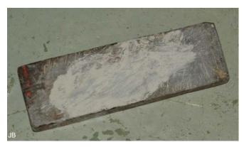
1) Whetstone. Although chisels are made of hardened and tempered steel, they wear in use. Proper maintenance of the tool is necessary. In normal use, occasionally simply use a fine stone or a sharpening steel for the blades.
