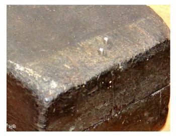
Also 2 nails, with their heads cut off, were driven into bottom for use on the bench to ensure footing during grinding.
