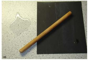
Pour some water on the work surface and put the sandpaper on it. By using a round stick or rolling pin going over it, we create a vacuum under the sandpaper so the paper will keep in place during sanding.
