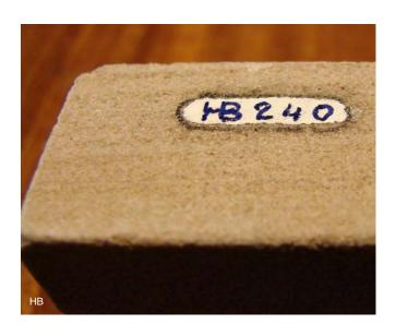
The number is applied using a permanent marker, and colour-fast markers with a point of 0.2 mm. After drying, it is finished with a layer of non-shiny Glitsa (a water bound lacquer).
