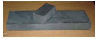
Slurry stone, used with slate to produce a "milky" grinding paste that gives a fast result with a dull surface as a result.
