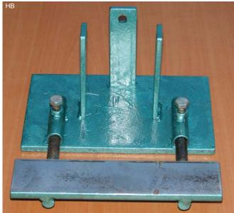
The Aldi (supermarket) grinder has 3 mounting holes of M 8. The stand for the grinder is made of some old iron from my junkyard. Make sure the tool rests perpendicular to the cutting surface. All that's missing now is the dust extraction. See also page 50 of the catalogue: http://www.beeldhouwwinkel.nl/catalogus 2011.pdf
