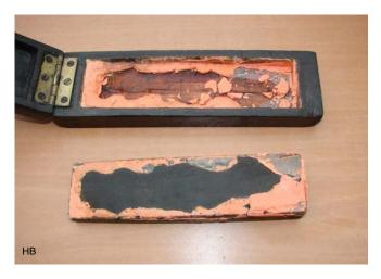
In English whetstone boxes you may find white- and redlead is mixed in. The reason for the red-lead powder is that it prevents the stone absorbing the linseed oil. Sometimes heated glue of bones is mixed with red-lead powder. I also found a form of Plasticine.
