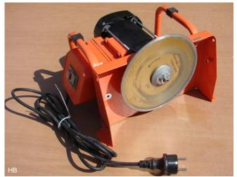
This is stripped to the base portion. The saw is also removed and after reaming of the bore of the abrasive disc to 25.4 mm it showed that it fits perfectly with sufficient ground clearance.
