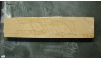
The drawing shows that the stone is a still a little hollow, therefore repeat the operation.
