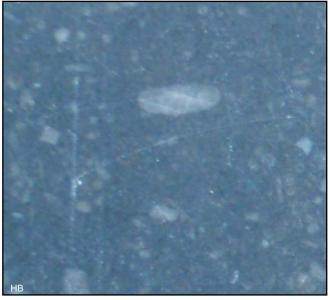
C800 = depending on material you can speak of polishing here, yet very small grinding marks are visible in raking light.
