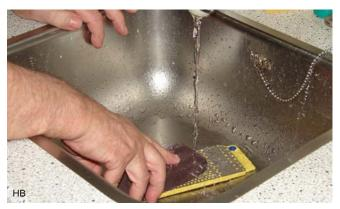
Here is the stone placed in the sink. This works uncomfortable because the stone begins to slide.
