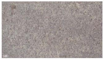
The back of this old Rouge du Salm (BBB) stone is very useful for grinding. Therefore, this is also flattened.
