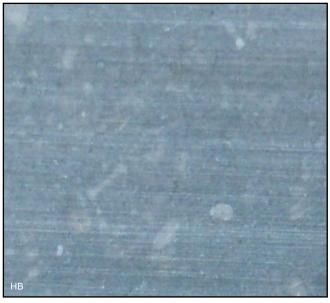
C320 = satin surface, grinding marks still visible in raking light.
