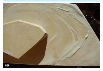
Coticule is a yellow compact metamorphic rock consisting of a large number of minerals. Density is 3.22 g/cm3. It occurs in layers of 2 mm to 25 cm. In the deep parts of the Basin of Vielsalm were in the Early Ordovician (about 480 million years ago) clay and silt deposited. Clay and silt have a grain size substantially smaller than the grain size of sand.
