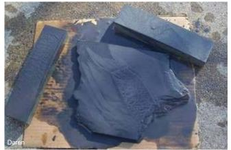
Others did this grinding with silicon carbide grinding bench stones and elbow steam. The stones were increasing in fineness. See <u>http://lumberjocks.com/Daren/blog/2835</u> The Spiegelberg sandstone is hand finished with a SiC waterproof sandpaper sheet with a grit of 600.
