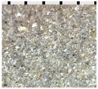
After 5 minutes grinding with 600 grit (USB microscope) The scale is 0.5 mm
