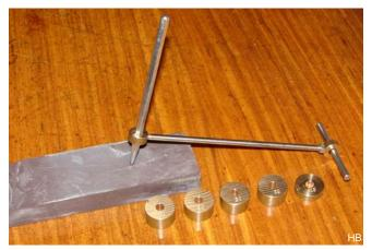
**Model 1** is a test probe with interchangeable weights. To do a test without weights the pressure to the needle tip is 50 grams. Can test from 50 grams increasing with 25 grams up to 250 grams.
