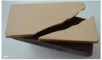
These broken coticule can be repaired virtually invisible by gluing carefully.
